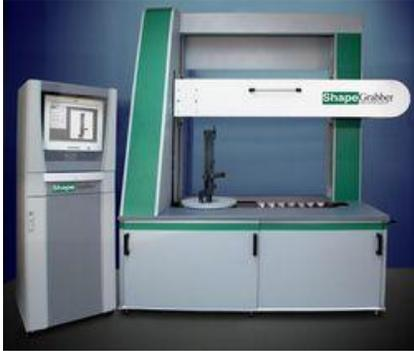
*ShapeGrabber Ai810 3D Scanner system with plastic radiator tank on rotary scan table (photo on left)*
